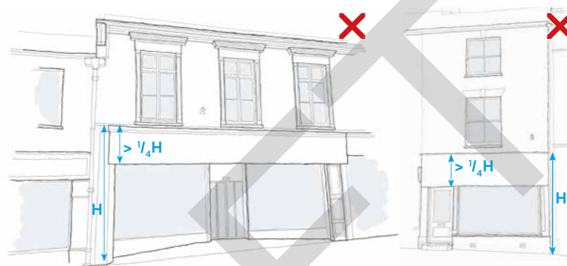
Loss of original features with the addition of a large sign. Oversailing the fascia, pilasters, and window heads.
